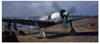
Focke Wulfe Fw 190A-8 Fighter – Radial engine of 1730 HP (some boosted to 2100 HP). Two 13mm machine guns in nose (400 rpg), two 20mm cannon in wing roots (250 rpg), two 20mm cannon in outer wings (125 rpg), one 550 lb. bomb or 300L drop tank on centerline rack. Speed on deck clean = 350 mph, with bomb = 325 mph. Combat radius with bomb = 120 miles, endurance = 45 to 55 minutes (drop tank would add 20 minutes or so but replaced bomb). Damage absorption - Fair. Dogfight agility - Poor.
